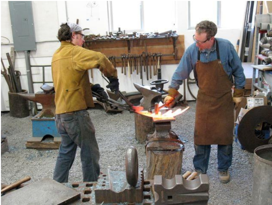
The artists cut the giant plant shapes out of steel and formed the steel by hand-using traditional blacksmithing tools.
