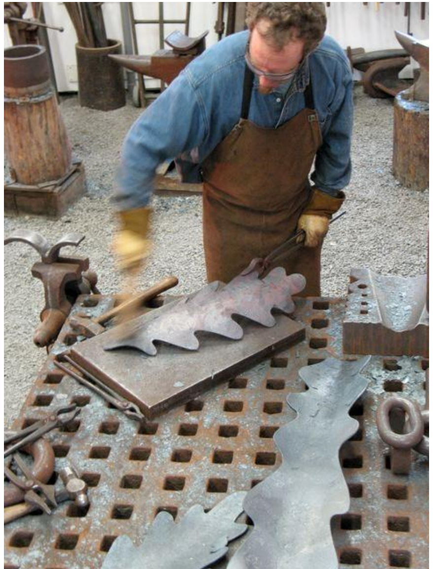
The metal shapes become softer when heated. Then they can be hammered and formed into curved shapes like real leaves.
